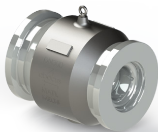
3X7H Range Hub End Connection Manufacturer's Pattern Face to Face Sizes 2"-42" Rating ASME Class 150 - 2500
